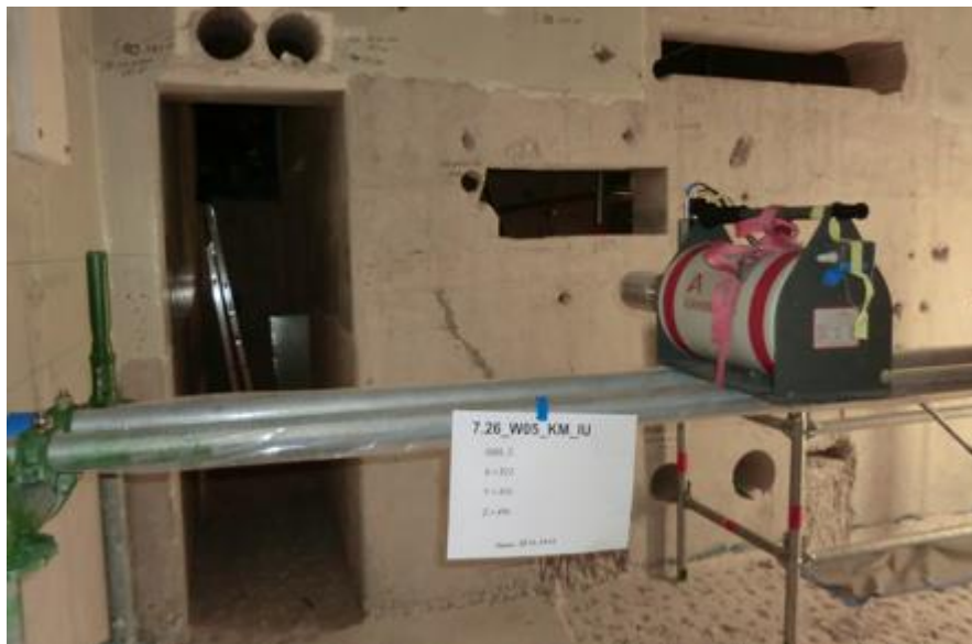
Figure 10: In-situ gamma spectrometer for decision measurements of buildings (Brenk Systemplanung GmbH)
