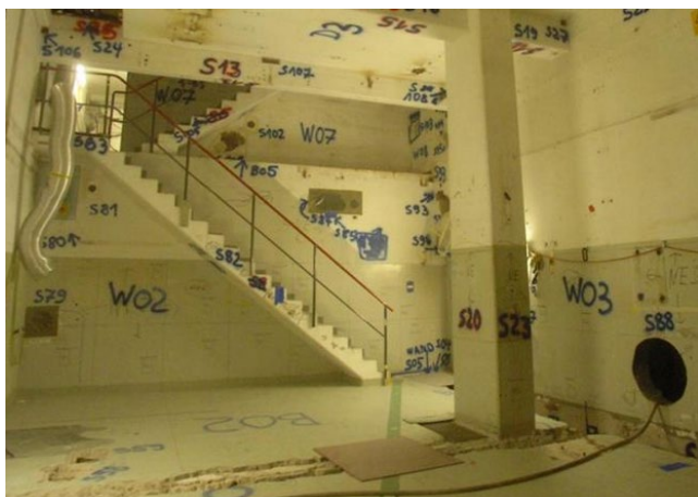
Figure 6: Room to be measured for clearance with sampling points (PreussenElektra GmbH, Würiggassen nuclear power plant)
