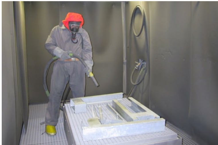
Figure 9: Media blasting of metallic components (PreussenElektra GmbH, Würgassen nuclear power plant)
