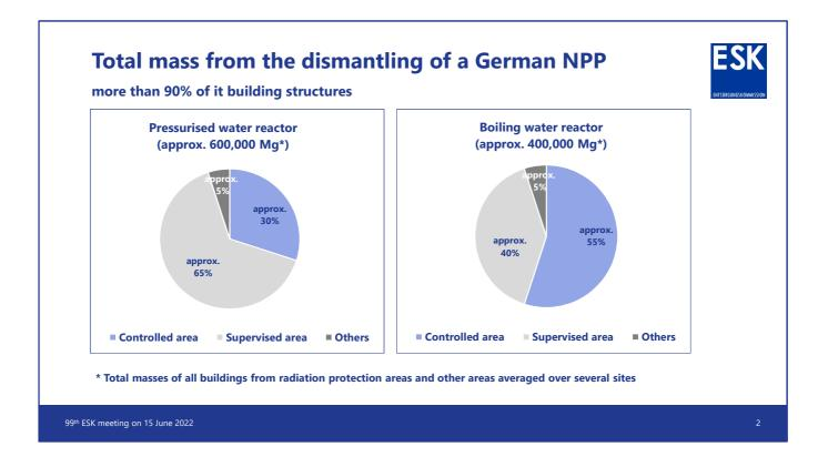
The total masses given here refer to the nuclear power plants to be dismantled in Germany. Some of the smaller plants already dismantled produced significantly lower masses. The dismantling of individual nuclear power plants commissioned in the 1980s, such as the Krümmel nuclear power plant (KKK), produced significantly larger total masses, without resulting in significant differences with regard to the percentages shown here.
